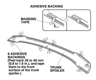
19. Remove the adhesive backing from seal B. Align the two clips and the stud bolt with the holes in the trunk lid, and install the spoiler. Apply pressure to the trunk spoiler over each clip until you hear a click. Do not apply excessive pressure.
