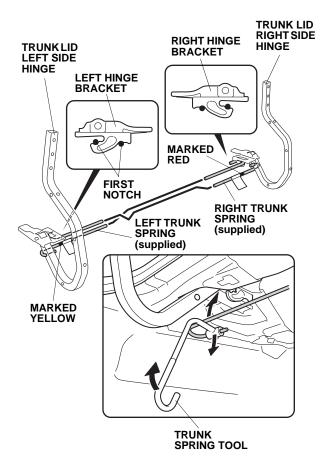
29. Reinstall the center clips onto the trunk springs.
