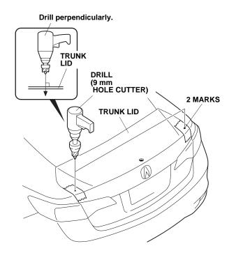
13. Remove the tape installed in step 3. Remove all burrs and metal shavings with a file, and apply touch-up paint to the edges of the holes.
