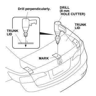
12. While wearing eye protection, drill two 9 mm holes at the marks near the outside edges of the trunk lid with a 9 mm hole cutter. Drill perpendicular to the trunk lid.
