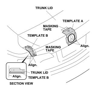
5. Using a felt-tip pen, mark two points through templates A and B as shown.
