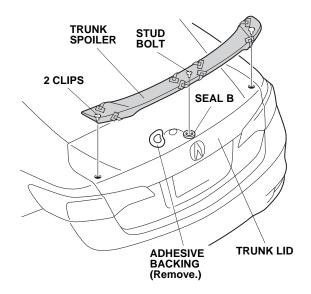
20. Adjust the position of the trunk spoiler so there is equal spacing on both sides.
