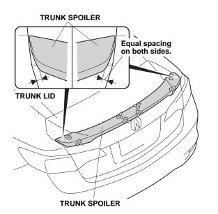
21. While applying light pressure against the trunk spoiler, carefully remove the adhesive backings as shown.
