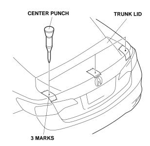
11. While wearing eye protection, drill an 8 mm hole at the mark in the center of the trunk lid with an 8 mm hole cutter. Drill perpendicular to the trunk lid.
