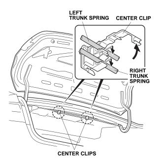
27. Put on heavy gloves to protect your hands. Use the trunk spring tool to remove the trunk springs from both trunk lid hinges. Pull the trunk spring tool slowly and carefully toward you. First remove the right trunk spring, then remove the left trunk spring.
