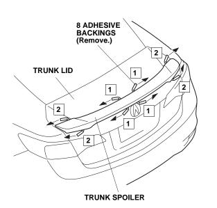
22. Using your hand, firmly press the trunk spoiler against the trunk lid.
